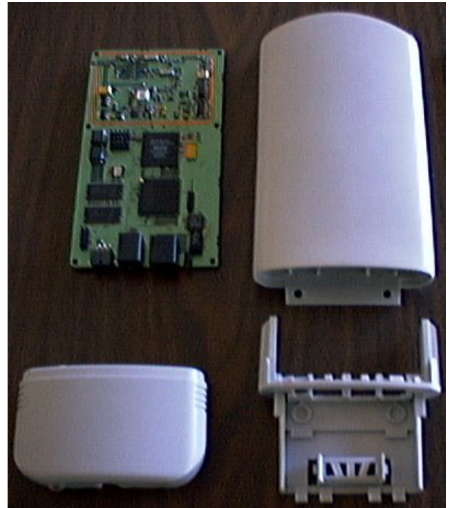
Elements of the Motorola Canopy. The lack of complex chips on the board is notable.
